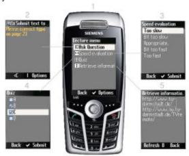
Figure 2. The *TVremote* Prototype running on a Siemens S65 mobile phone
